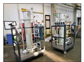
made of plastic material so that they can not be attacked by ammonia and other aggressive contact fluids.
