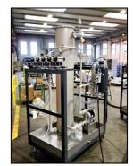
The plant is supplied key in hand, complete with control and safety instrumentation, everything managed by an electric panel equipped with a PLC, which guarantees the highest ease of operator / machine dialogue.
